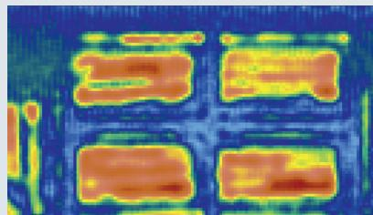
**Types of defects:** air pockets and electrolyte distribution
