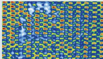
**Types of defects:** impact damage and delaminated top layer
